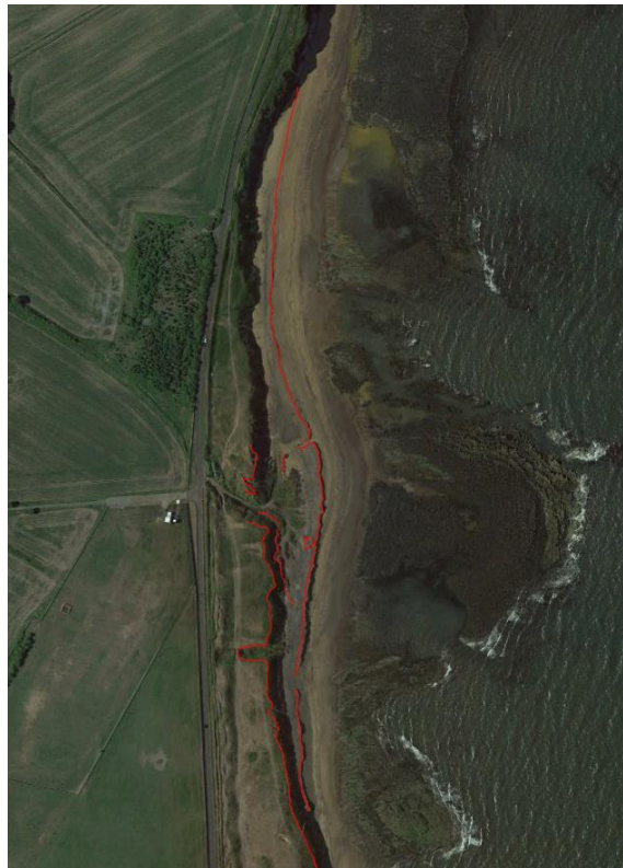
Figure 3 – Baseline cliff top survey (North)
